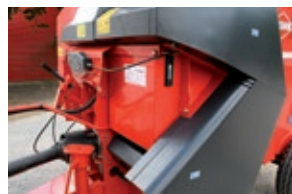
45 L/min -1 (12 gpm) hydraulic power unit
