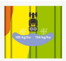
This new application is available as option on the CCI 1200 terminal. It enables to apply two different application rates, meaning to control the left and right metering unit of a fertilizer spreader separately.
