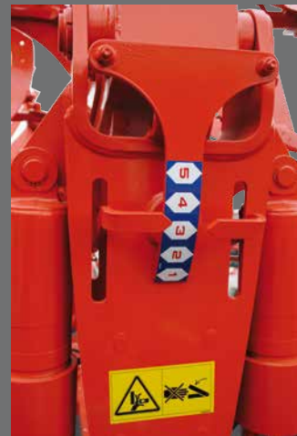
3. Offset : by mechanical tie rod or hydraulic cylinder (as an option) makes the inter-tyre adjustment from 1.15 to 1.60 m. A gauge visible from the tractor cab facilitates setting precision.
