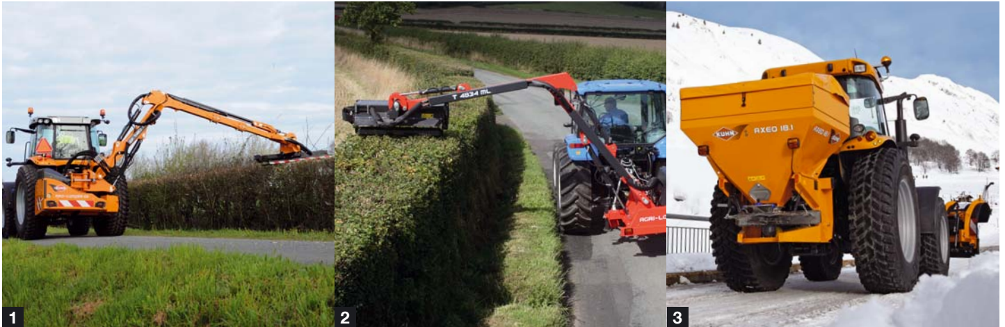
1 & 2. Hedge and grass cutters (left or right) with a horizontal reach of up to 7.40 m 3. Salt and sand spreaders
