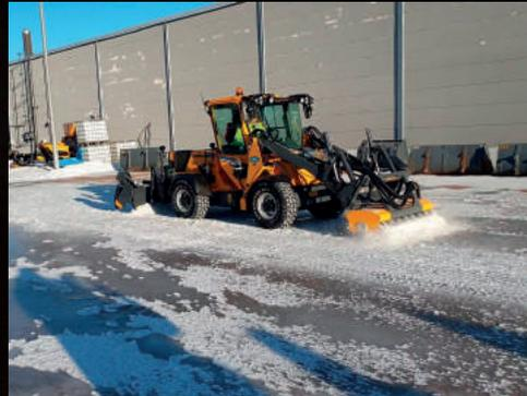
**MC4-Hydraulic** crushing of ice from parking area
