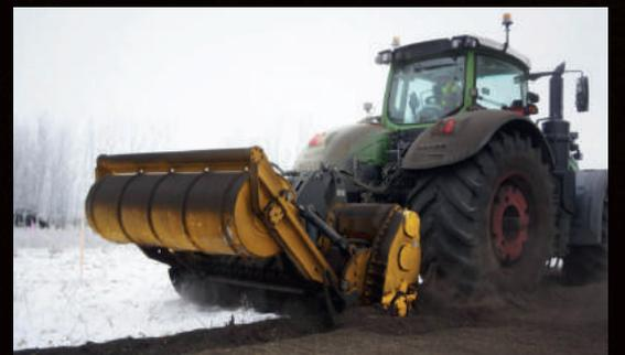
**MJF** Crushing of frozen soil from pipeline construction
