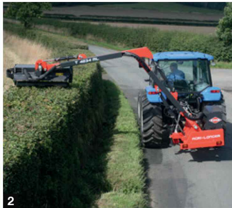
1 & 2. Hedge and grass cutters (left or right) with a horizontal reach of up to 7.40 m 3. Salt and sand spreaders
