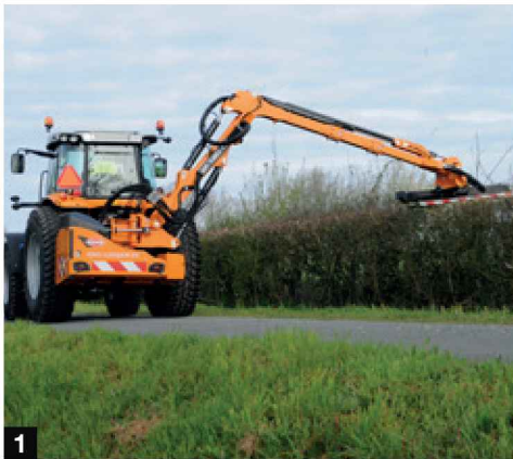
1 & 2. Hedge and grass cutters (left or right) with a horizontal reach of up to 7.40 m 3. Salt and sand spreaders
