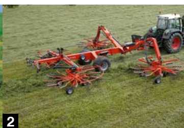
1. Mounted single-rotor rakes 2. Semi-mounted four-rotor rakes 3. Belt mergers 4. Tedder-rake combinations
