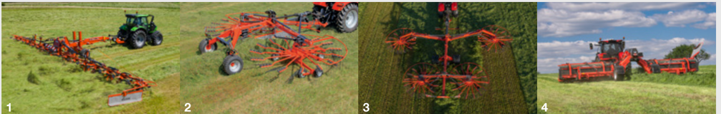
1. Gyrotedders up to 17 m - 2. Twin rotor gyrorakes - 3. 4-rotor gyrorakes - 4. Belt mergers up to 13 m
