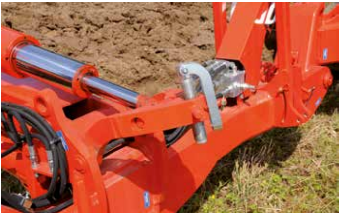
1. Levelling : by independent left / right crank screws for extra precision.
