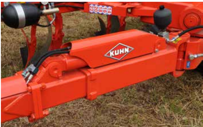
3. Offset : by mechanical tie rod or hydraulic cylinder (as an option) makes the inter-tyre adjustment from 1.15 to 1.60 m. A gauge visible from the tractor cab facilitates setting precision.
