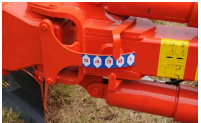
3. Offset : by mechanical tie rod or hydraulic cylinder (as an option) makes the inter-tyre adjustment from 1.15 to 1.60 m. A gauge visible from the tractor cab facilitates setting precision.
